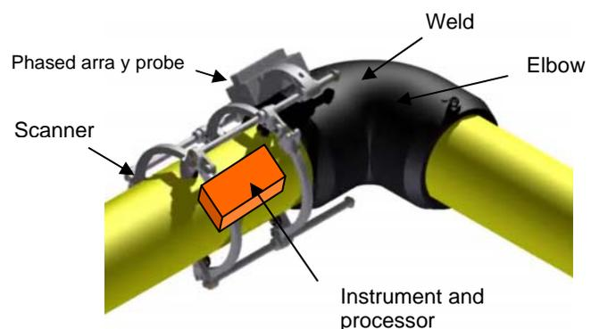
*Schematic of proposed TestPEP ultrasonic inspection system*
